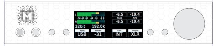
To enter the one of four parameters menu shown on the display, press one of the four buttons located on the left and right side of LCD display. When the value is ready to change it is back-lit with blue colour. To change the value rotate the knob until you see the option / value you need. Press the knob (or the same button) again to leave the menu.
